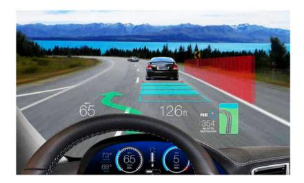
The Data Apps and Analysis subteam is also developing an AR Windshield, which entails displaying live information about the vehicle using a heads-up display that is projected onto the windshield. This project aims to also integrate with all subteams' autonomy divisions, so that features including displaying the car's optimal path on the windshield can also be added in the future.
